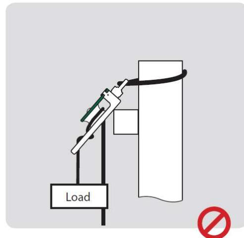
3. The OX BLOCK is designed for multi-braid synthetic ropes (maximum size 5/8" (16mm)) and should not be used with wire ropes or natural fiber ropes.
