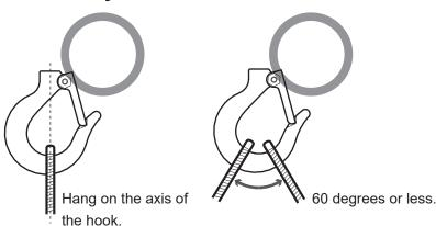
Avoid the dangerous hooking method shown in the following diagrams.
