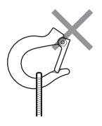
The holding object or the sling is not hooked in the correct position.
