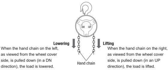
This product is designed for a rated load to be hoisted by pulling the hand chain with a force shown in the "Pull to lift load" table below or less. If an excessive load is applied, the overload limiter will operate. In this situation, immediately stop the operation and lighten the load.
