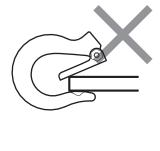
The load is applied at the tip of the hook.
